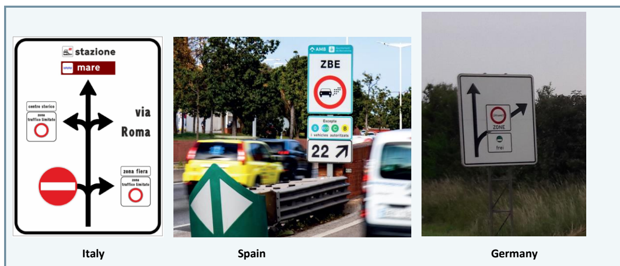
Figure 7: Examples of advance warning signs
