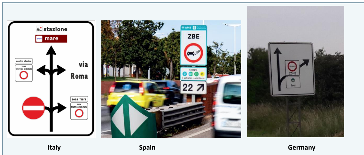
Figure 7: Examples of advance warning signs
